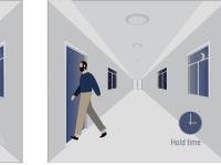
The sensor turns OFF light automatically after the holdtime when there's no motion
