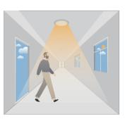
The sensor turns light ON when motion gets detected.
